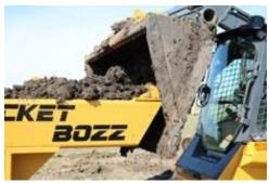
Hard Mount Loader Tool Operation - Position the loader bucket in front of the BUCKET BOZZ's hard mounted loader tool and with a slow downward motion scrape out the impacted material.
