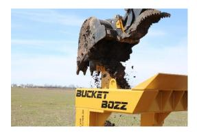
Excavator Tool Operation- Using an excavator, reach the boom and bucket over the BUCKET BOZZ to the excavator bucket cleaning tool. Slowly lower the bucket down on the cleaning tool scrapping the bucket clean.
